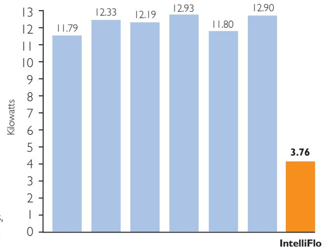
Data shows results of comparative energy use tests between IntelliFlo and six common pool pumps. IntelliFlo consumed between 68% to 71% less energy in every case. In actual use conditions, savings may be significantly larger.
